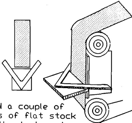
Weld a couple of bars of flat stock to the tool rest, flanking the platen & extending behind the belt, i.e., no more blades getting sucked between the rest and the belt.
